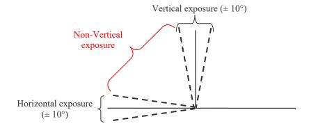
• The real durability of a product depends on a large number of parameters, including, among others, the quality and preparation of the substrate, exposure (environment, climate, exposure angle), graphics maintenance, and degree of pollution.
