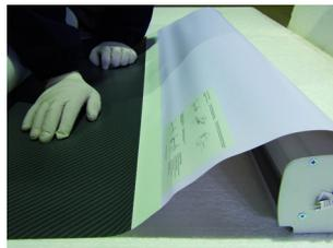
Once the graphic is applied to the tape, firmly press down over the full width to ensure proper adhesion.
