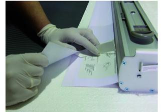
Partly expose the double-sided tape and start applying the bottom end of the graphic.
