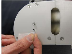
Remove the pin in order to slide the graphic into the base. Be careful to maintain the graphic and the base so that the winding is done properly.
