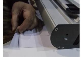
Remove a part of the double-sided adhesive tape and start applying the bottom of the graphic.
