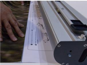
Keep applying the graphic until it is fully bonded.
