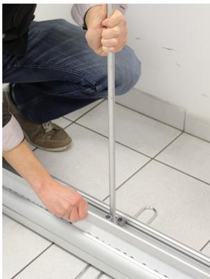
Remove the graphic from the base while holding the mast.
