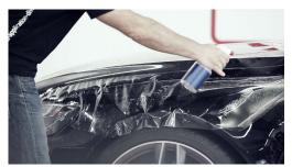
> Spray the vehicle body to be protected as well as the adhesive-coated side of the BODYFENCE with the HEXISGEL or soapy liquid (PULVERISAT or SHAGSPRAY) (FIG. 03). This will enable a better positioning of the product on the vehicle.
