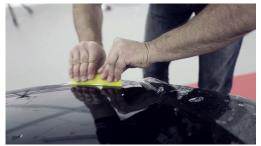
> To ensure that the squeegee glides easily, spray the HEXISGEL or soapy liquid (PULVERISAT or SHAGSPRAY) onto the BODYFENCE film. Then apply it, holding the squeegee at 45°. Press firmly to adhere the film to the surface and remove the application liquid. (FIG. 05)
