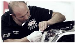
> Firmly apply the film with the squeegee to the edges, rounded sections and adjacent or opposite faces of the body. (FIG. 10)
