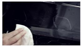
> Place absorbent paper on the SHAGFENCES squeegee. Apply pressure to the cut edges to remove as much as humidity as possible. (FIG. 09)
