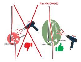
> Stretch the vinyl over the substrate so that the film touches the peaks only. (FIG. 08)
