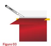
> Peel off 10 cm (4 in.) of the liner. (FIG. 03)
