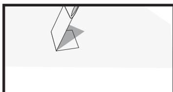
Using a TESA® 7476 adhesive tape, or similar, apply it to a surface of 2.5 cm x 5 cm (1 in. x 2 in.) plus some overhang material for easier removal. Fold and promptly tear it off perpendicularly to the substrate surface. No traces should remain on the ripped-off adhesive tape. Repeat this process in several places.
