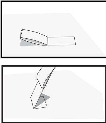
Using a TESA® 50110 adhesive tape, or similar, apply it to a surface of 2.5 cm x 5 cm (1 in. x 2 in.) plus some overhang material for easier removal. Fold and tear it off with one quick pull perpendicular to the substrate surface. The film must generate a certain resistance during its removal. Repeat this process in several places.
